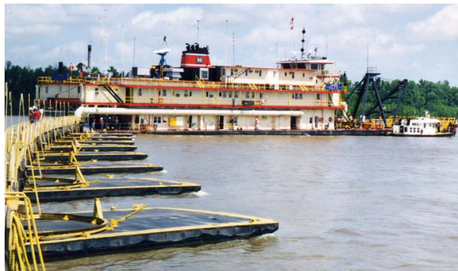
Hydraulic Cutterhead Dredge with Pipeline on Pontoons
