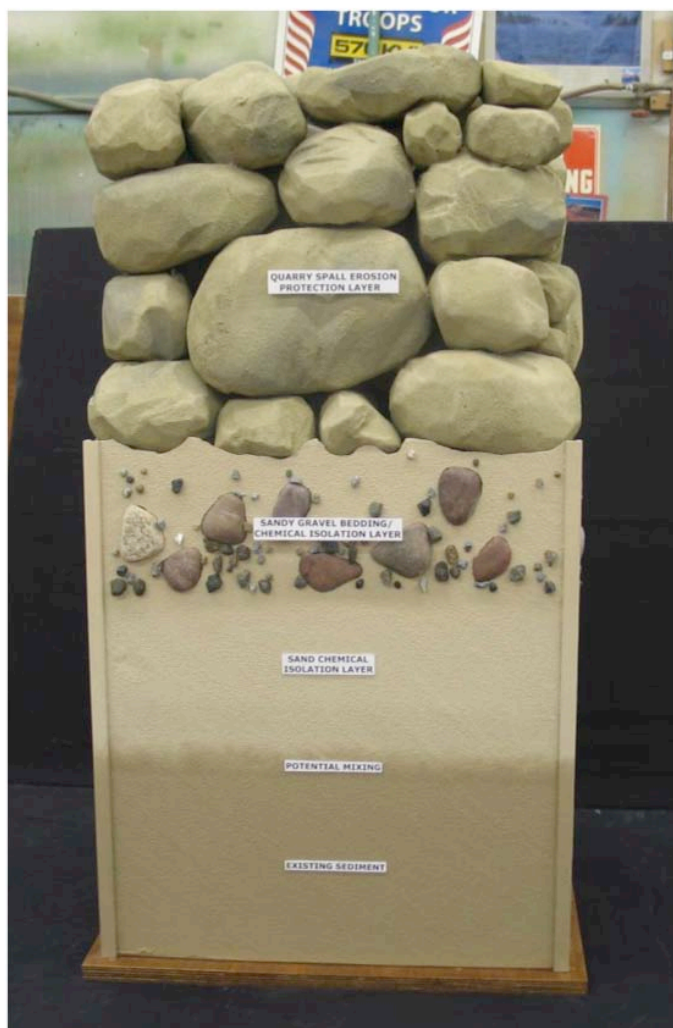
Model of Typical Armored Engineered Cap Cross Section
