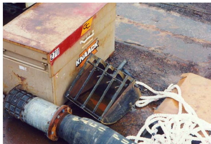
Diver-Assisted Suction Dredge (photo shows nozzle of hose)
