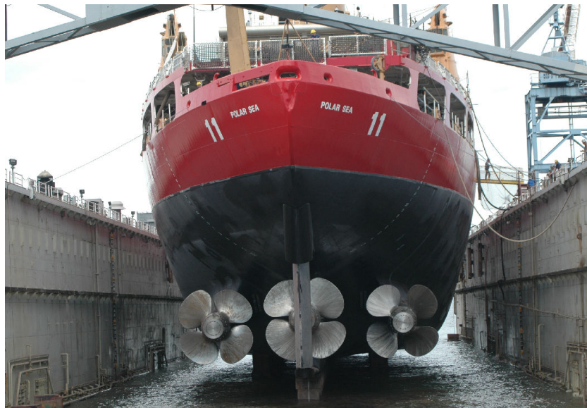
Figure 13. Polar Sea in dry dock showing propellers and rudder (area 2)
