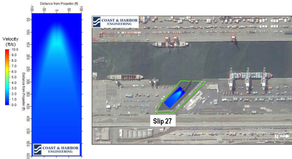
Figure 18. Pattern of near-bottom velocity of Tug Hunter D in Area 3
